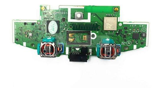
• Is the main brain of a controller, in this case this one only have two joisticks , some thancistors, vibrators and a microchip.
