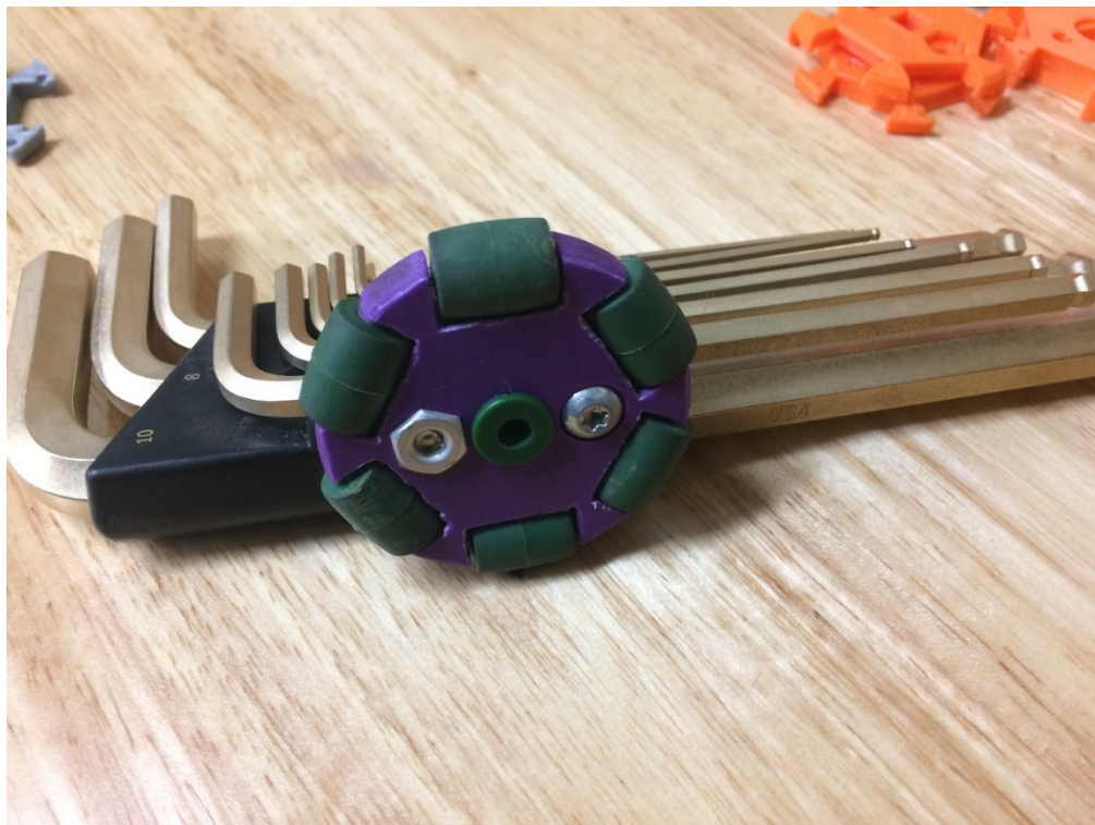
Image 5: Assembled wheel using the clamshell hub design and round high strength shaft inserts
