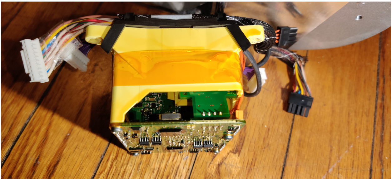
Figure 18: Side view of the Sensing Unit, with the cast IMU holder attached to the module
