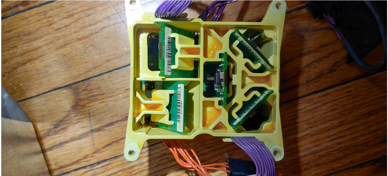
Figure 17: Top view of the Sensing Unit, with the cast IMU holder keeping the IMUs from moving out of position
