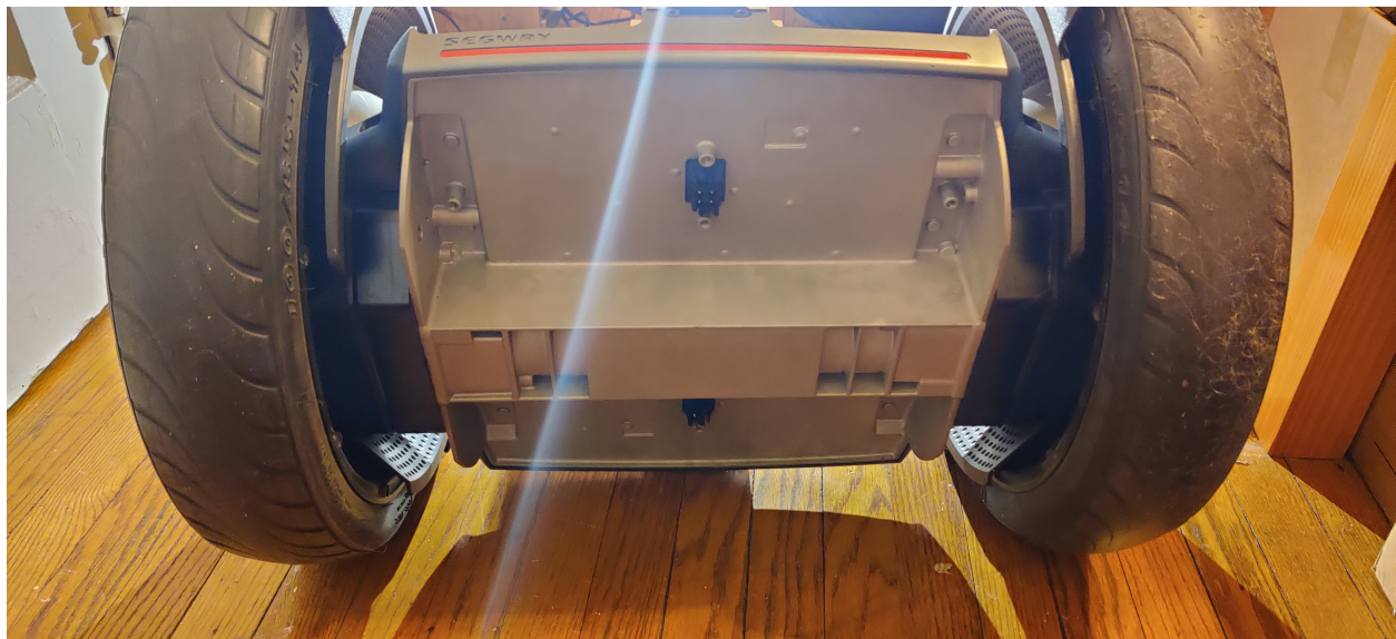
Figure 9: Dual Steel Battery Bays for the Segway. Each battery connector supports 74V connections and I2C communications
