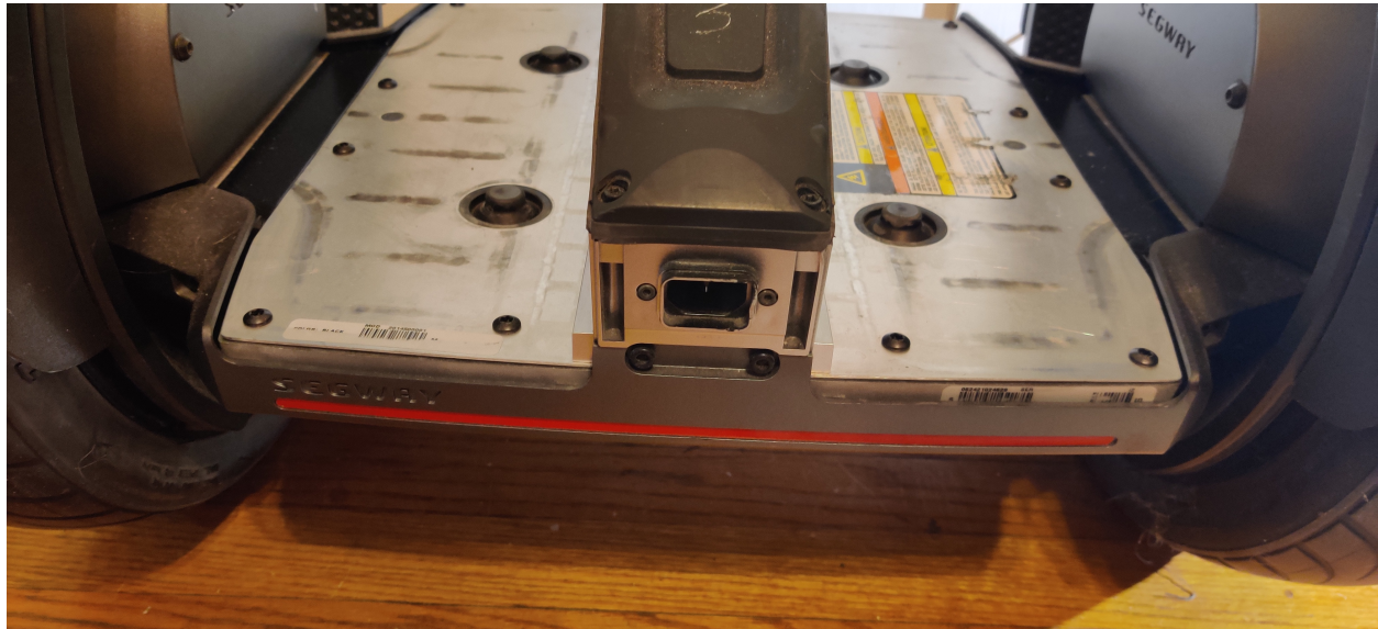
Figure 8: Segway charging port (rear) with rubber trim pieces removed
