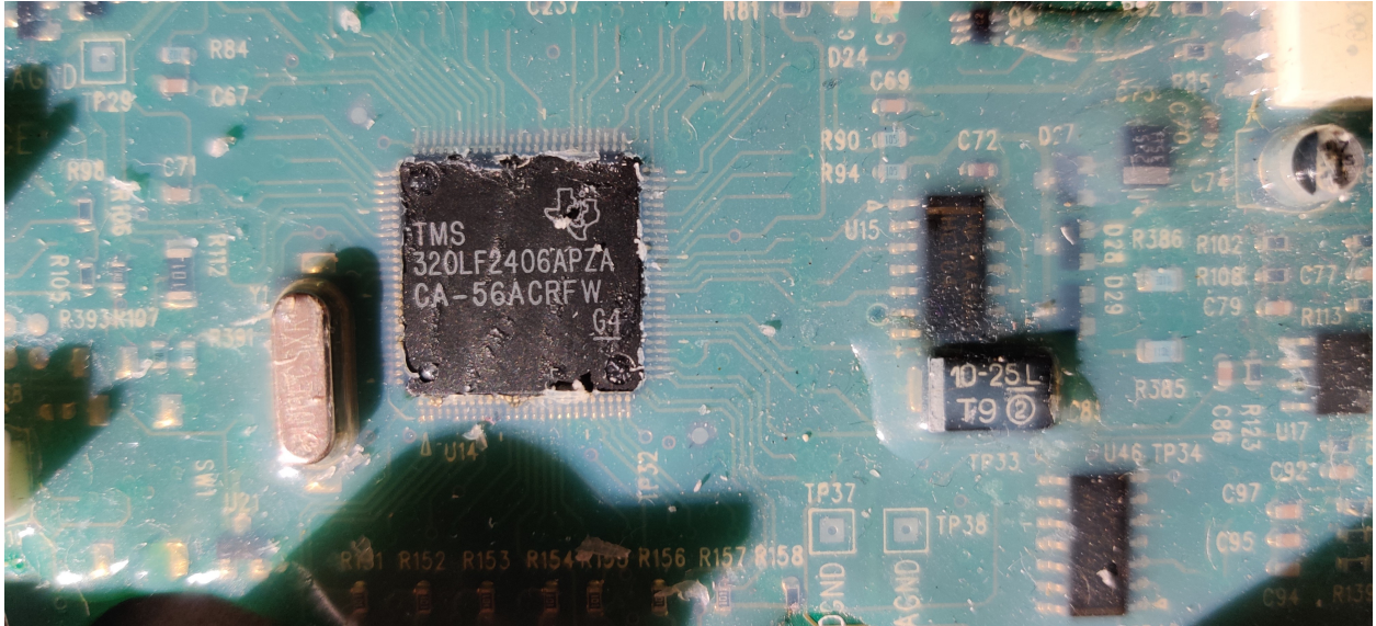
Figure 1: Close-up of a Primary Control Unit DSP (Component 25 ) and it's respective traces covered in Conformal Coating
