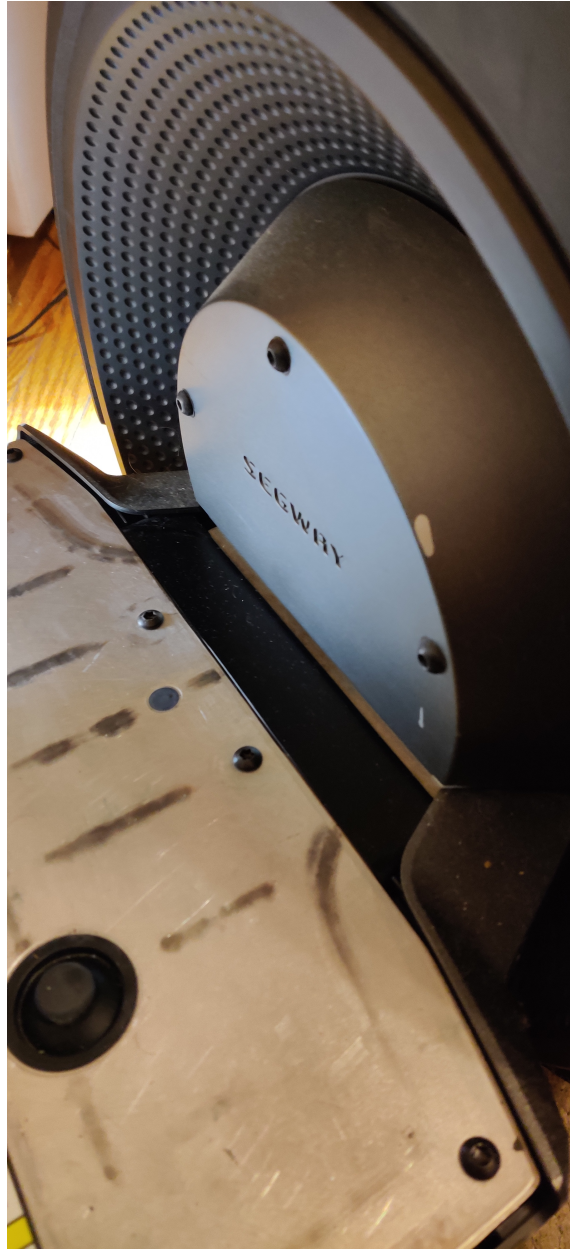
Figure 7: Side wheel trim piece firmly mounted to the platform
