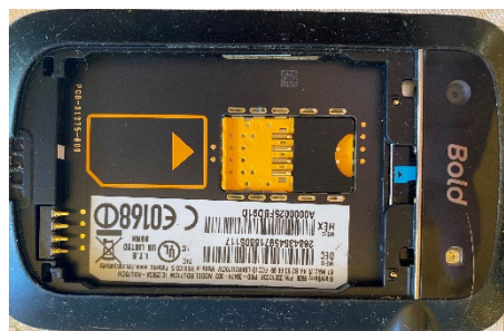
Figure 1.3 Identified Version from Label, Serial No., Model
