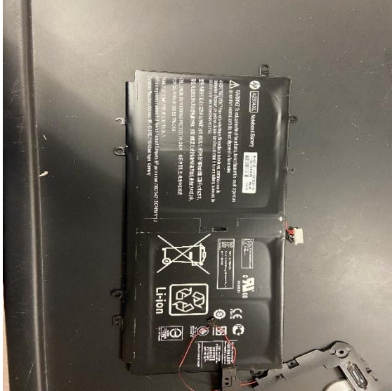
Figure 24-cell 51Whr 7 Ah lithium-ion polymer battery
