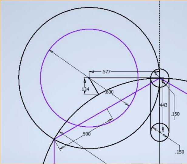
"Slot" for the pin on the drive gear.
