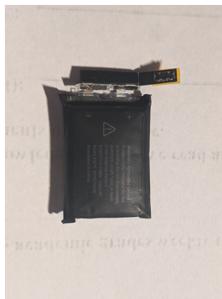
Fig-4(The Lithium-Ion battery, swollen and the reason why the watch stopped working.)
