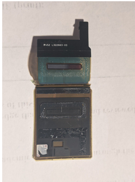
Fig-3(The back of the LED display and the cable connection from it.)
