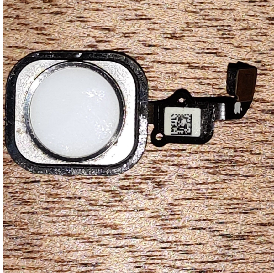
The sapphire button and steel ring, as well as the ribbon assembly are pictured above.
