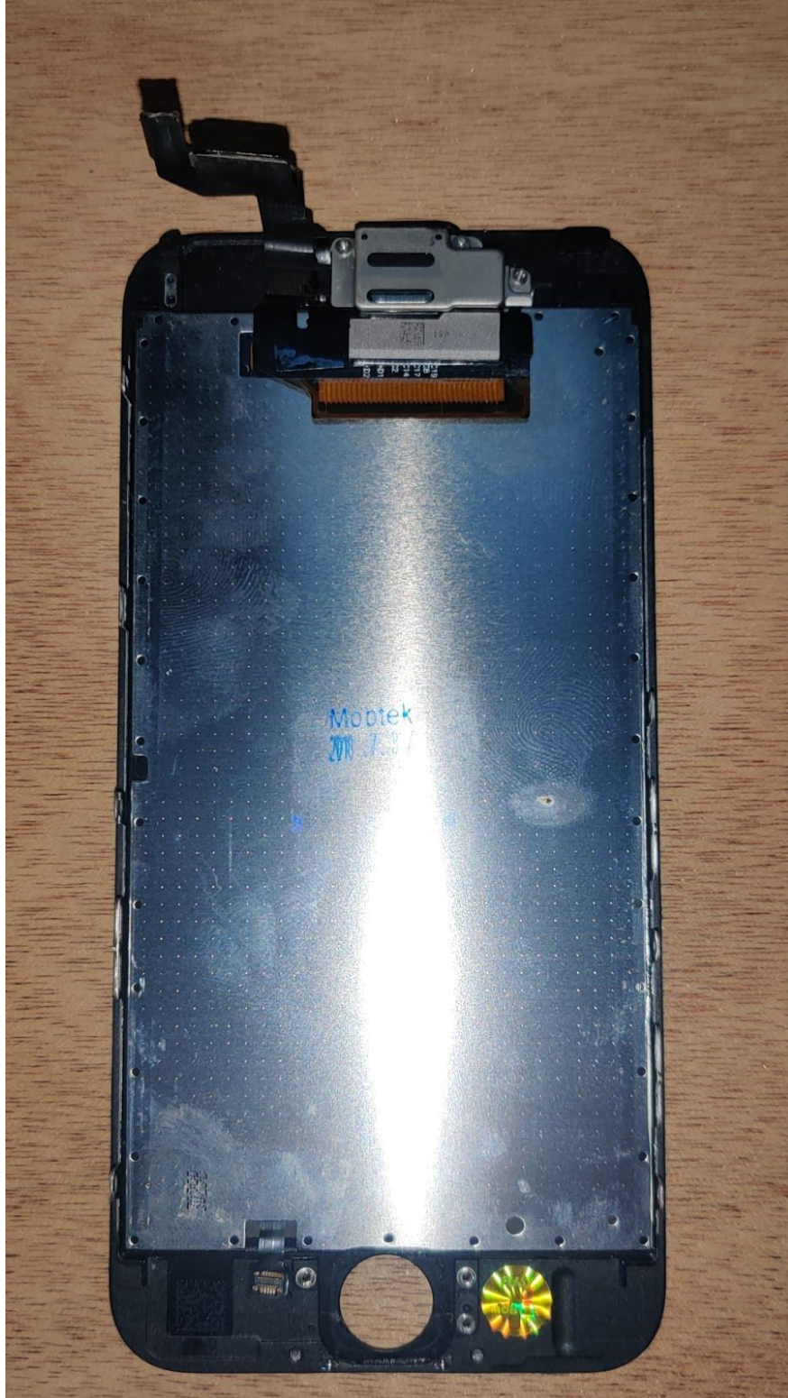
The home button flex connects at the bottom left corner and runs up behind the lcd shield to the digitizer cable.
