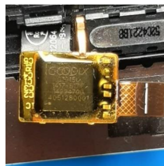
Figure 8: This 5-point touch controller converts touch input from the capacitive touchscreen into digital data. It supports 5 touchpoints at the same time (18)
