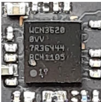
Figure 9: This IC enables network features like WLAN, Bluetooth, and FM Radio. It takes input from the CPU and then outputs to the antennas. (17)
