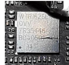
Figure 5: Qualcomm WTR1625L Transceiver
