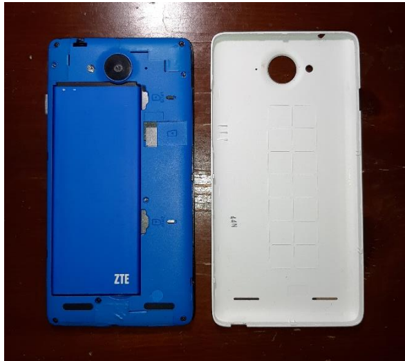
Figure 10: The plastic back is removed easily, showing the removable battery. There are also two SIM trays and one microSD card slot.
