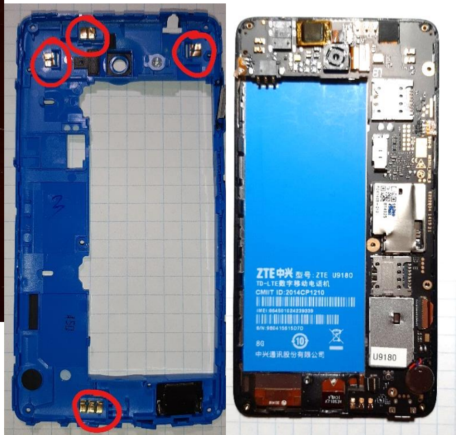
Figure 11: We found the blue shroud has metal contacts that are embedded in tape on the outside. We think these are radio antennas.
