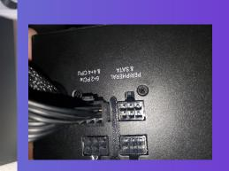
You may ask how do you get power to all of your components and why do you need a power supply and why isn't there something smaller well The computer power supply changes alternating current from a wall socket of mains electricity to low-voltage direct current to operate the processor and peripheral devices. Several direct-current voltages are required, and they must be regulated with some accuracy to provide stable operation of the computer.
