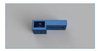
The first two configurations are meant to be put on sides without motors. These have a slot in the middle or the side for the locking collar to go through. They also have two screw holes that attach to the metal. To use the Aligner, simply put a locking collar in the slot, screw it in, put the axle through, and tighten. In the slot there is a ridge for the set screw to go along easily.
