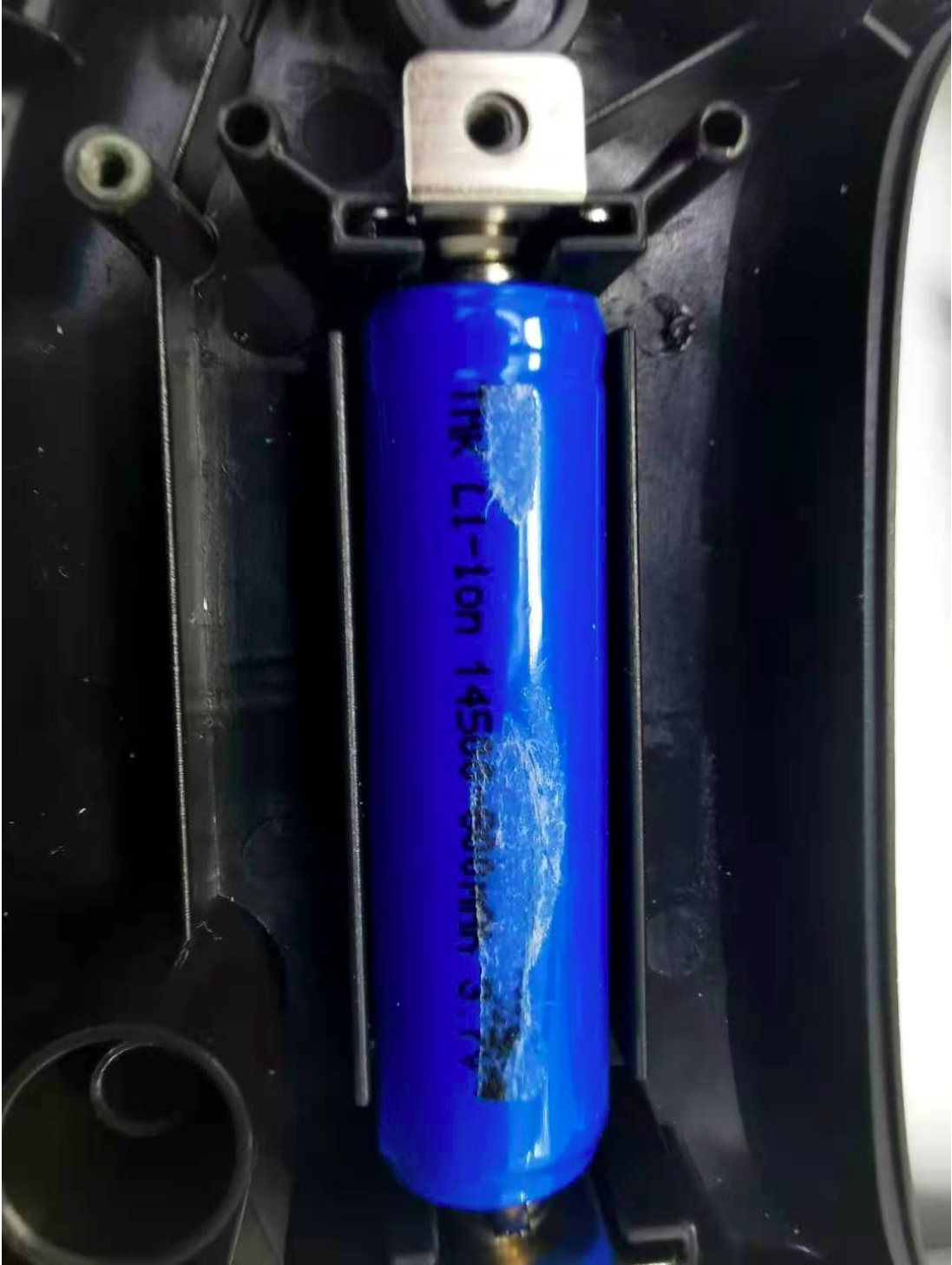
This is a chargeable battery under the motherboard, it can be connected to a charger on the outside.
