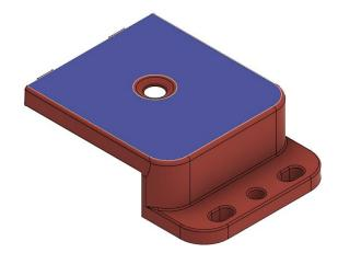
After the cap was extended forward, the portion of the encoder lid that would be attached to the original mounting holes would be extruded downwards to the base of the encoder (about 13.6mm).
