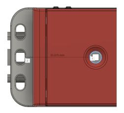
Afterwards, I measured the size of the slots to replicate it to the new mounting hole of the model. Using a c-channel CAD model, I made sure the holes were the correct distance from the center hole. In the end, the holes aligned perfectly to the center, holding symmetry.
