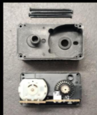
Figure 2.4 Cover piece removed, exposes the internal components
