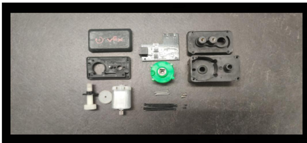
Figure 2.10 Motor fully disassembled | screw count: 12
