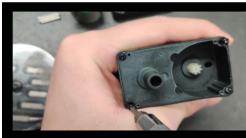
Figure 2.3 Unscrewing the middle cover of the motor
