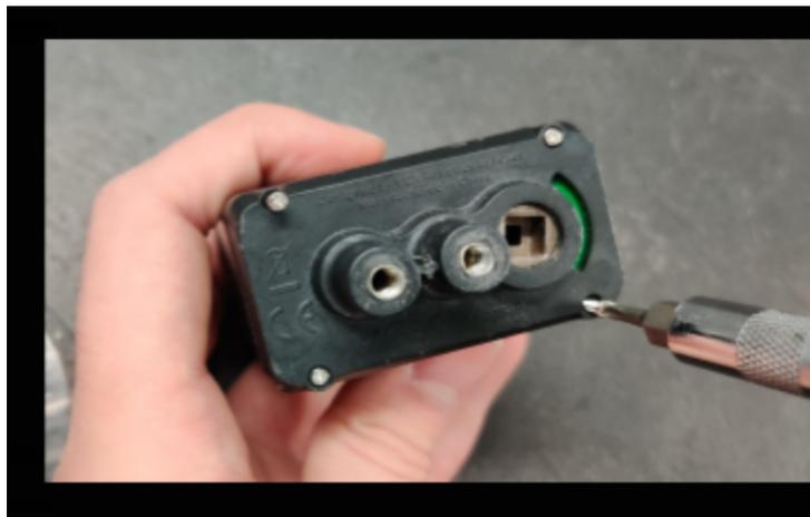
Figure 2.1 Unscrewing the top cover of the motor
