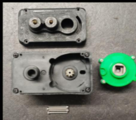
Figure 2.2 Parts found after removing the bottom cover
