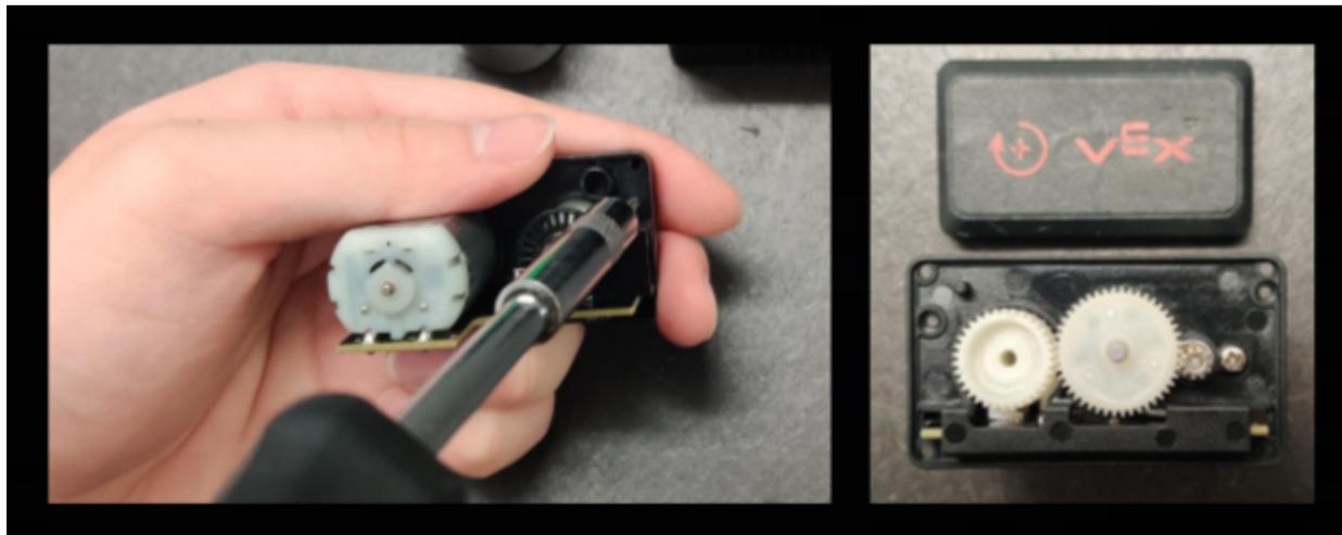
Figure 2.6 Unscrewing the bottom cover of the motor
