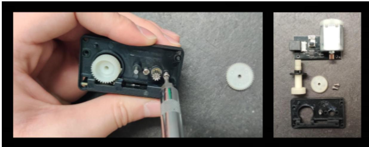
Figure 2.8 Unscrewing the DC motor from the frame
