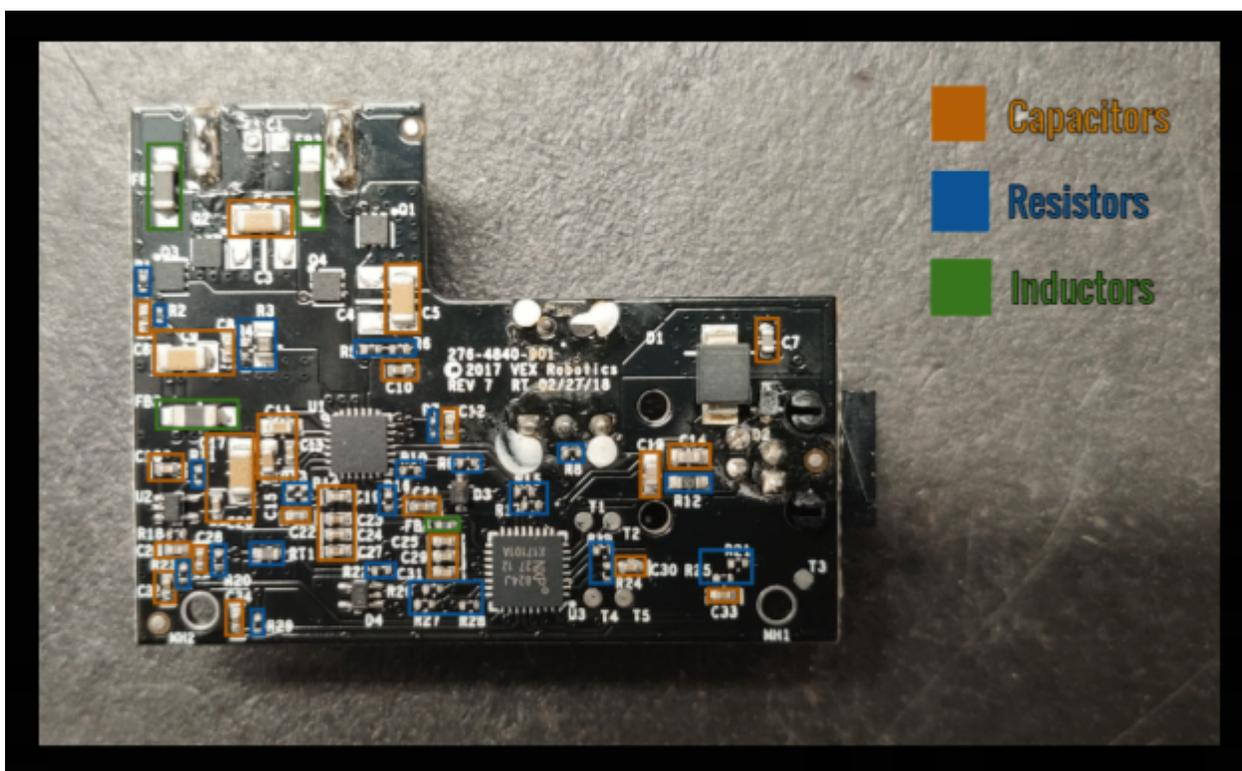
Figure 3.4 Components on the back side of the mainboard
