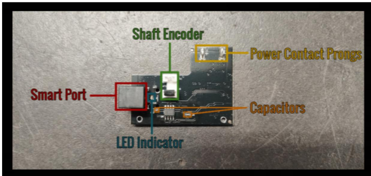
Figure 3.3 Components on the front side of the mainboard
