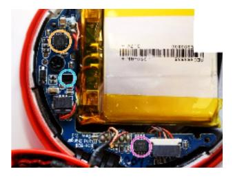
Here the orange circle is the BQ2407:y Li-Ion Battery Charger and Power-Path Management IC, the blue is the battery fuel gauge (BQ27425: Battery Fuel Gauge) and the pink is the PCA9536: s I/O Expander
