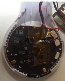
component we researched was the bq27425-G2 fuel gauge which provides fuel gauging to the Lithium batteries. The next part we found and researched was the BQ2407:y Li-Ion Battery Charger and Power-Path Management IC. This component is basically connected to the lithium batteries and it manages the power flow through the headphones. Next we found the TCA6507:
