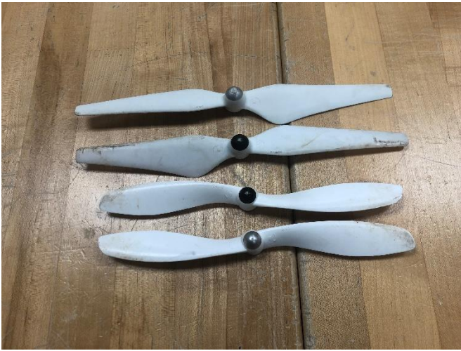
Figure 5. First, I twisted off the propellers, each of which is uniquely specific. There are opposite front/back models along with duller versions for the rear.
