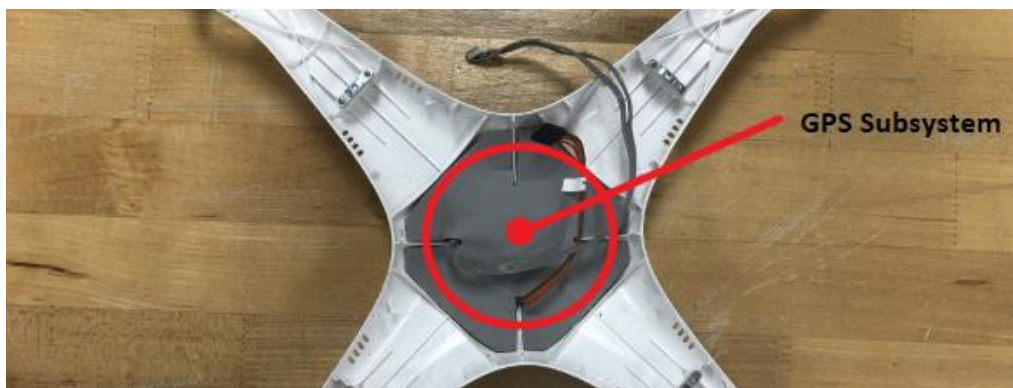
Figure 9. The only component linked to the top drone case is the GPS unit, which connects to the landing gear's compass module.
