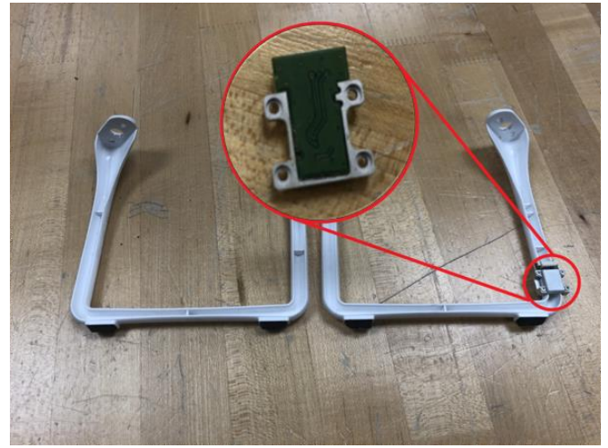
Figure 6. I then removed the landing gear, which houses a component of the GPS: the compass module. It needs physical separation distance from the motor vibration.
