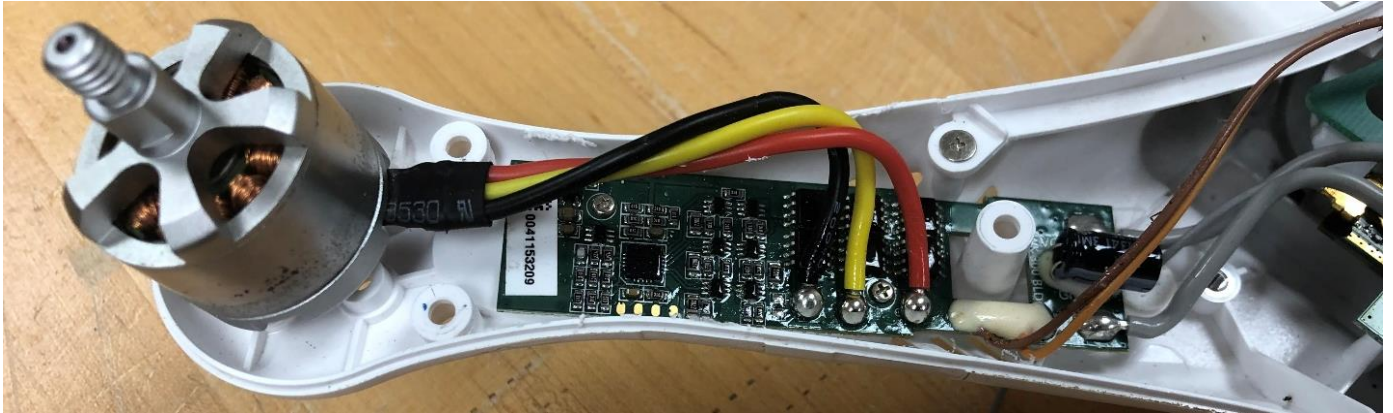
Figure 18. There are four identical motor/propeller subsystems, which consist of power delivery and a motor control system that converts power & data to motor output.
