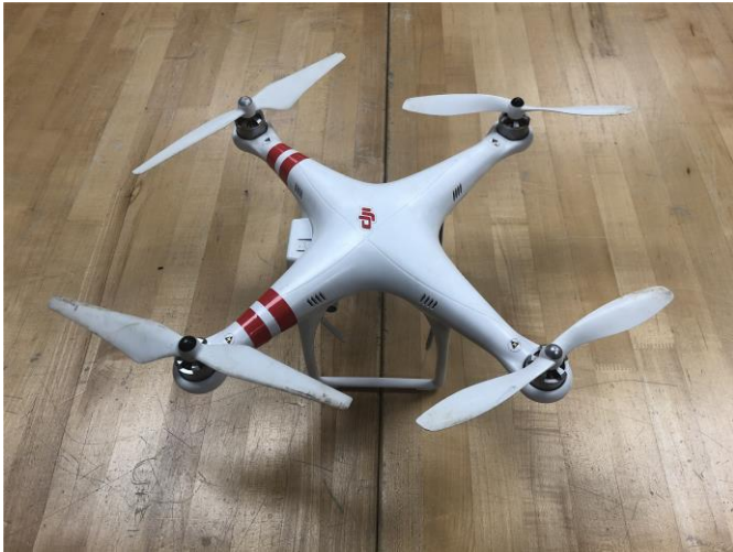
Figure 2. This is the constructed DJI Phantom 1 drone. It is a rigid-base quadcopter with four independent propellers for flight control.
