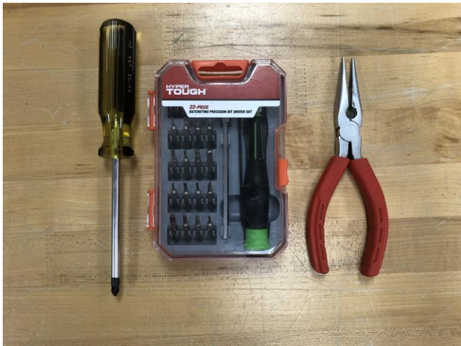
Figure 3. I used various tools for the deconstruction process: a Phillips-head screwdriver, a 3/32" hex screwdriver, and pliers. There were several screw standards across the build.
