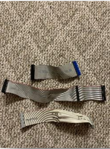
These are the ribbon cables
