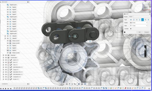
Adjust the position of the joint so that the chain link will be in line with the other links.
