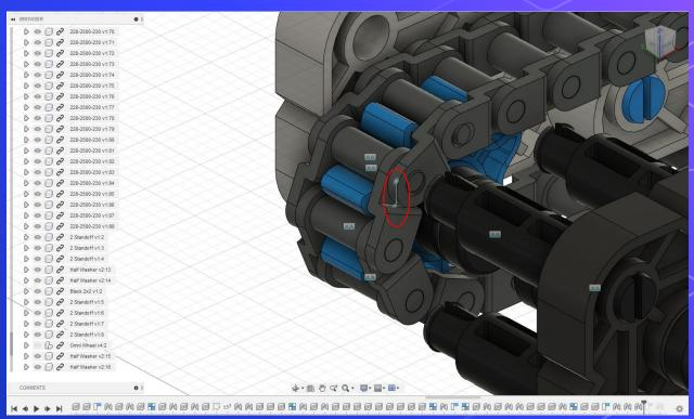
Now use the move tool, but in a new mode. First, switch the move type to point to point. Second, select the circle part of the sprocket not in line for the origin point. Third, select the sprocket circle in line. This will move the piece, much like a joint, except it won't constrain it.
