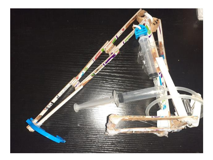
This is a hydraulic crane, it can move vertically by the purpose of its function, for it to move horizontally, you must do it manually. Its purpose is to lift a container up with stuff in it. The pressure from the water pushes the handle up gives a up and down motion.
