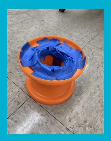
In our second design, we added another hub on top of the first hub to add more capacity. The new problem was that the bags that went to the bottom were out of reach. The only way to get the bags out was lifting the holder which would make all the bags fall out. This happened because the bottom was left open.
