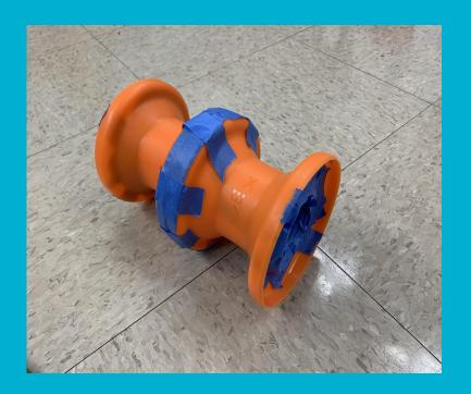
In design 3 we wanted to make a holder that could take out bags from both sides. To do this we made the same ring setup on the other end of the hub. This design worked because it could fit a good amount of bags and the way you use the holder was easy. We needed to improve this design because it did everything we wanted it to do but the rings were coming off when you tried to pull out a bag.
