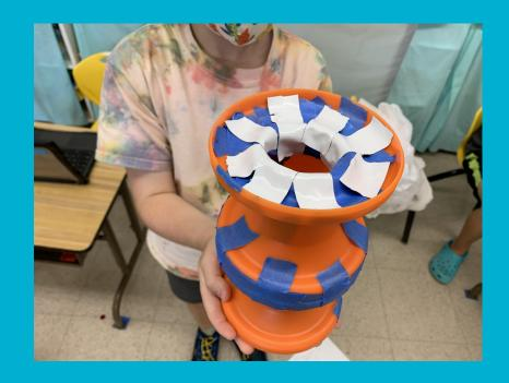
For design 5 we took off all of the painters tape and only used gorilla tape. A problem we encountered was that the gorilla tape kept getting stuck on the plastic bags. The gorilla tape tore the plastic bags and made the ring fall off the hub. It didn't look very nice either.
