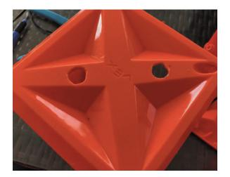
• Drill hole on the side for the cables
