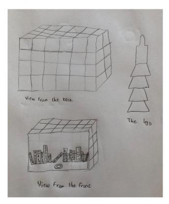
For the box, we used the cubes from 2019 - 2020 VEX Tower Takeover and hot glued each of the cubes together. Unfortunately, the glue wasn't strong enough to keep the cubes completely stuck together, so we added x-shaped square beams from 2016 - 2017 VEX Crossover. Using the holes already in the beams, we drilled in screws that connected the different cubes so by doing this, we made the walls, floor, and roof more stable.
