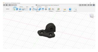
This is essentially a normal pillow block, except one of the mounting holes was moved in a way that lets one screw screws in both holes, making it much more secure.
