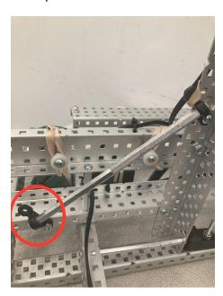
We have used many bracket braces on our robot, to strengthen the structure. While using normal pillow blocks is doable, we wanted to come up with a stronger design, one that can still have two screws in a C-channel.
