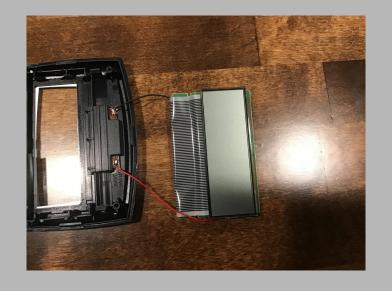
The display screen for this particular calculator, measuring ½ by 2 inches, for a total of 1 square inch. This screen can display up to 10 characters, not including a decimal point.
