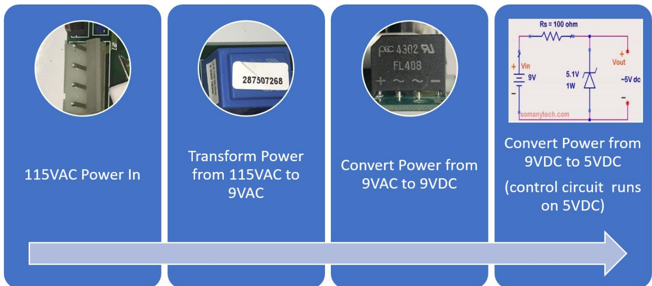
Flow Chart 2: Power Flow Chart for Coffee Machine
