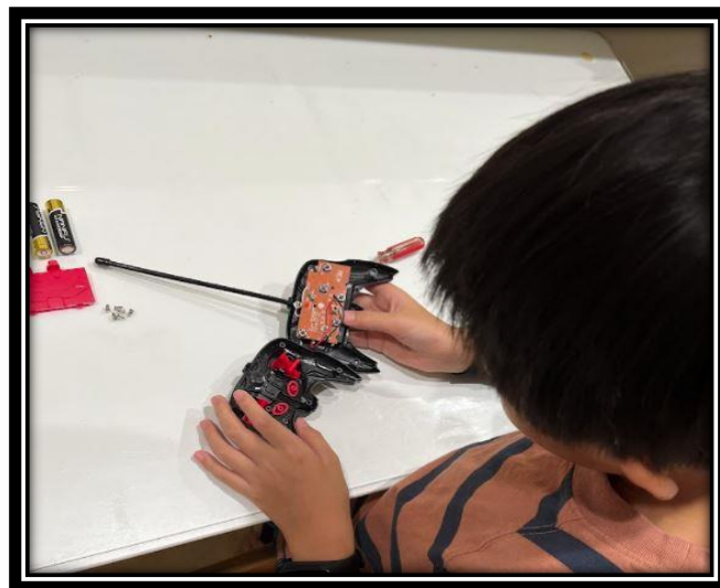
Figure 5 : Removing the outer casing to get access to the internal circuit board
