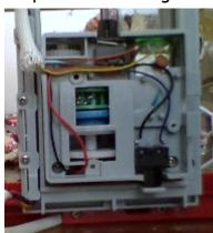
5. To take apart the gear box. I unscrewed 3 screws to get the top part off.
