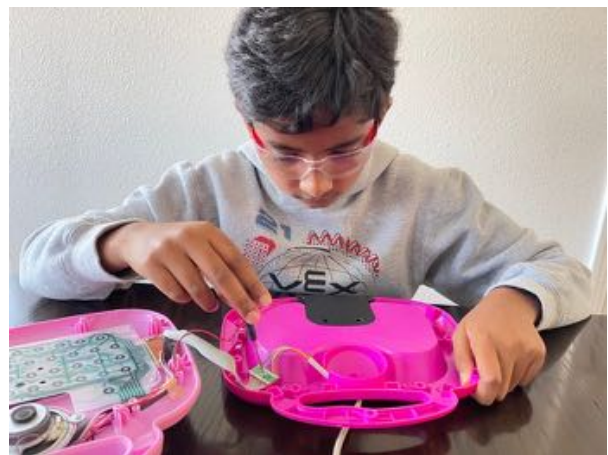
Step 7: Disconnect mouse wire
