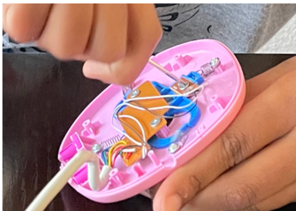
Step 8: Dismantle the mouse.
