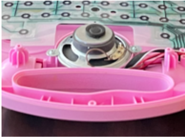
Step 9: Remove the speaker and button
