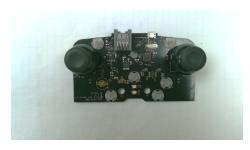
Radio transmitter: Sends radio signals to the robot brain, so we can control the robot.
