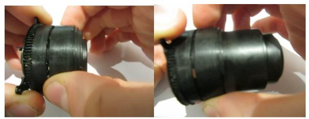
And when the part containing the shutter is removed, light can pass through the lens:
