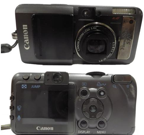
To deconstruct the camera, I used the Rolson 9-in-1 precision screwdriver. The camera screws have PH000 heads
