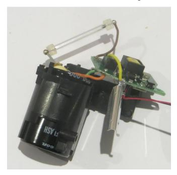
The capacitor has a capacitance of  $200\mu F$ . When the flash is required, the capacitor is charged then suddenly discharged through the glass tube. The glass tube contains xenon gas, which produces light when the electricity flows through it. This discharge creates the sudden bright flash.
