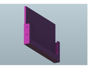
The License Plate Mounter has two screw holes on both of its sides along with 9 holes on the bottom, for increased adaptability depending on a bot's constraints. Two screws are effective in securing this lightweight part, making it easy to remove and relocate on a bot if necessary.
