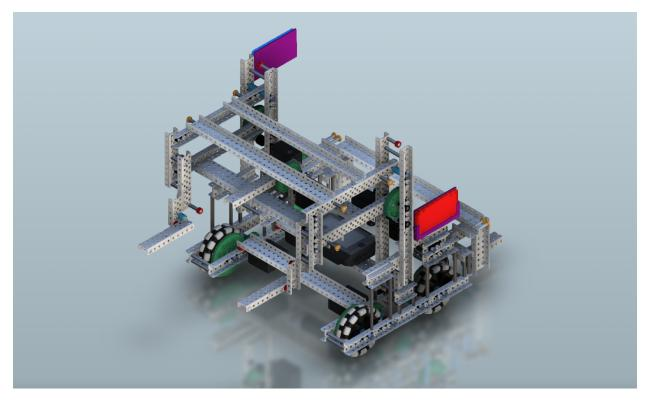
On our current robot for this year's game, Tipping Point, attaching the license plates directly onto the outside of the supporting bars for the 4-bar lift would cause the bot to exceed sizing constraints. Furthermore, replacing our two license plates without the License Plate Mounters takes over a minute. However, with the License Plate Mounters attached within the current dimensions of the bot and in convenient locations, we do not run into this issue.
