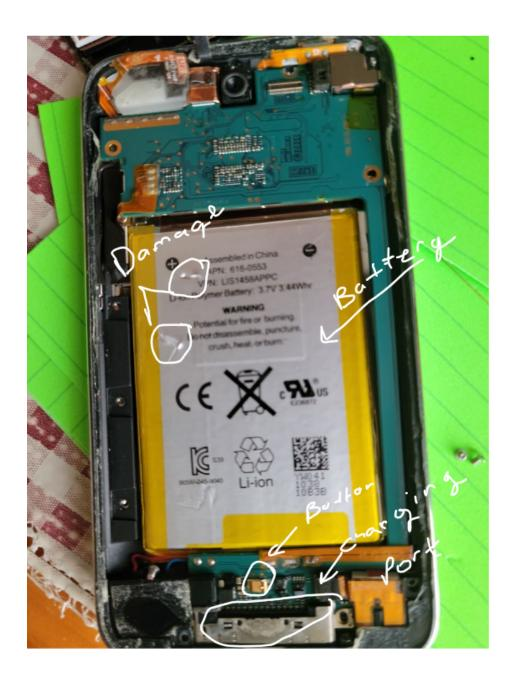
Afterwards, we removed the logic board (the blue green circuit in the above picture). We found the speaker on the bottom right and removed it. We also found the volume buttons and found that a deformed piece of metal was stopping it from working accurately (*mystery solved*).Next, we removed the rear camera and found a snaking orange cable. We concluded that it was the power cable.
