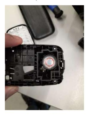
The speaker allows the phone to convert byte-stored sound into actual sound, and then play the sound to the user, which means that sound effects can be added to games, and radio can be played, as the speaker then converts the radio waves into sound, and this is crucial for calling as well, as then the user can hear what the caller is saying, and can appropriately respond depending on what is said.
