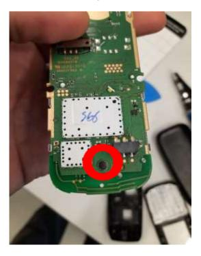
The microphone allows the user to give sound input to the phone, which can then be converted into bytes by the microphone, and then transferred. The microphone is crucial for handling voice calls, as it allows the user to speak to the caller.
