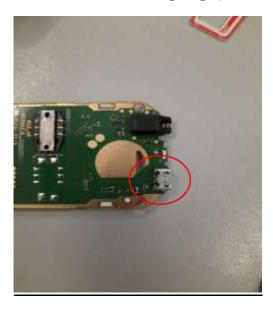
The micro-USB charging port means that when the phone's battery runs out, the battery can be recharged using a micro-USB cable. This means that the phone's battery does not have to be replaced as soon as it runs out, because it can be refilled, decreasing consumer costs and increasing sustainability.
