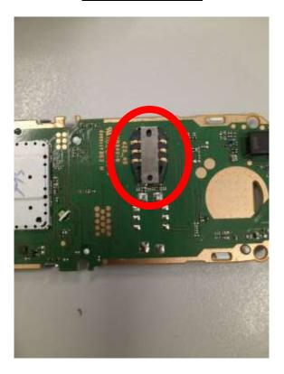
The SIM card slot allows the phone to use a SIM card, without which calling and messaging are not possible. This would make the phone practically useless, as it only has a small variety of games to play, and those are not the main function of the phone. The main function of the phone is communication, which required a SIM card and therefore a SIM card slot.
