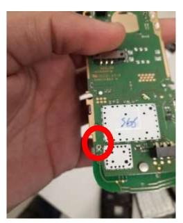
The antenna cable allows the phone to communicate with antennas, which allows it to play radio channels, as it can pick up their radio waves and convert it into sound.
