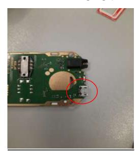
The micro-USB charging port means that when the phone's battery runs out, the battery can be recharged using a micro-USB cable. This means that the phone's battery does not have to be replaced as soon as it runs out, because it can be refilled, decreasing consumer costs and increasing sustainability.
