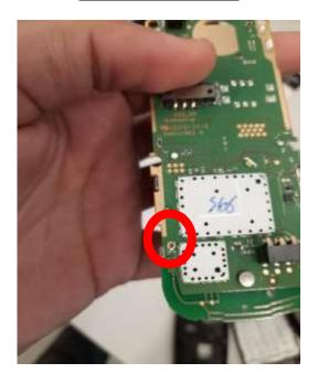
The antenna cable allows the phone to communicate with radio towers, which allows it to play radio channels, as it can pick up their radio waves and convert it into sound.
