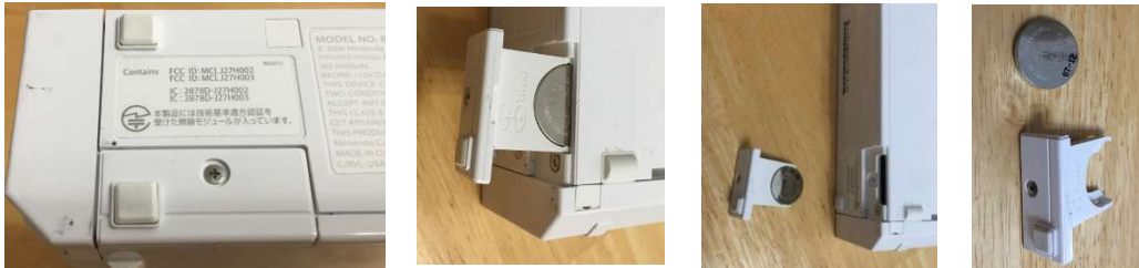
Figure 3.1: Removing Screwed socket
