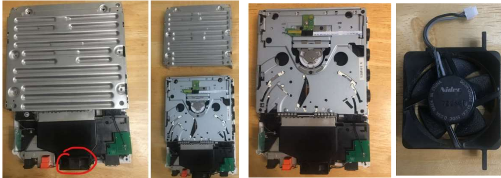
Figure 3.7.1: Removal of the metal cover
