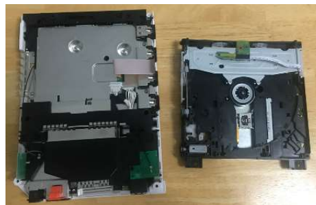
Figure 3.9: Removal of the Optical Drive
