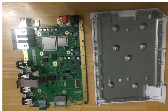
Figure 3.12: Removed Motherboard from the case
