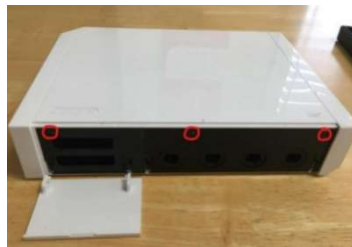
Figure 3.2: Remove the white cover flap
