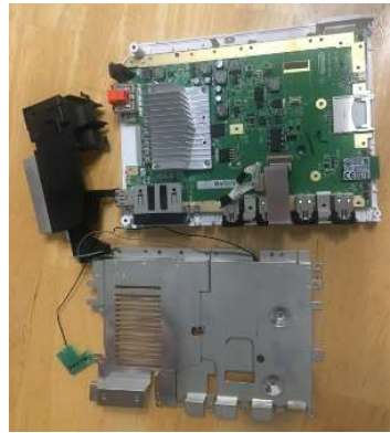
Figure 3.11: Removed motherboard cover
