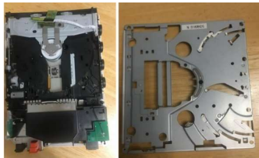
Figure 3.8: Removal of the Optical Drive Lid
