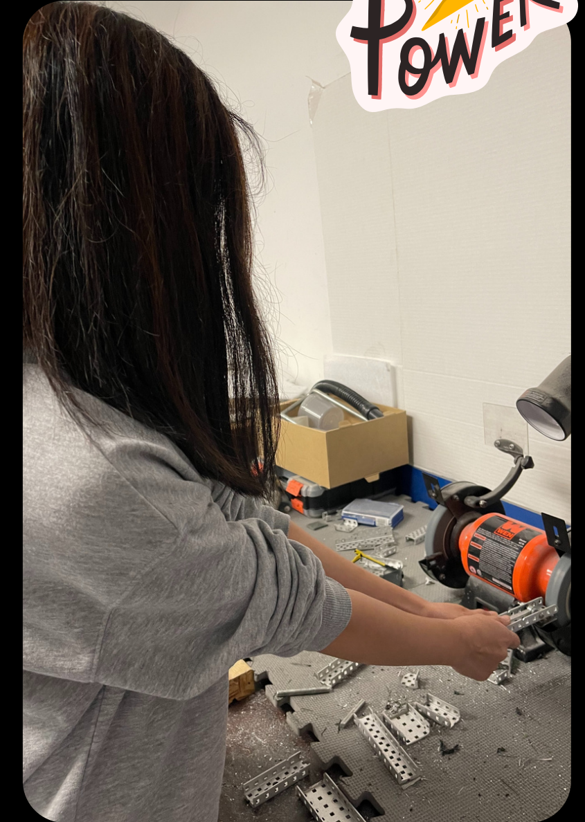
Priscilla grinding off excess debris from a c-channel
