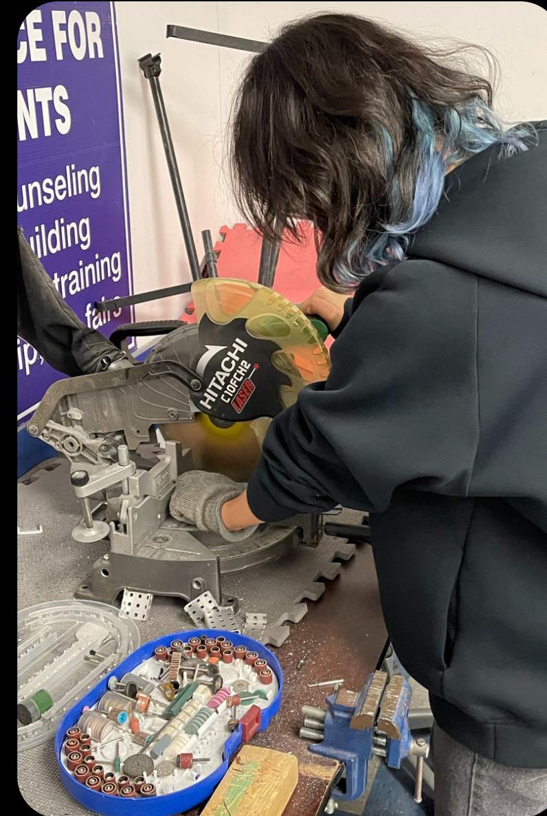
Priscilla grinding off excess debris from a c-channel
