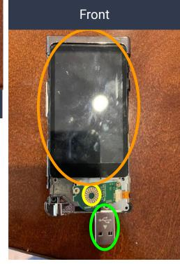
Most of the main electronics, including the motherboard, battery, and USB, have been uncovered, but none have been taken off yet. The camera, for example, is still hidden under the camera frame.
