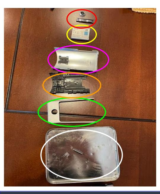
We started off just researching the Sony Bloggie, and we decided that the best thing to do was to take out all of the structural components. The buttons are plastic and rubber. The screws and connectors were hard to take out because they were small, and it was difficult to remove them without any damage.
