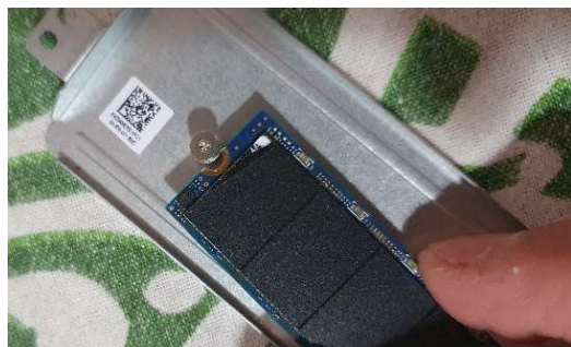
Left: Hard drive with memory units (black) showing, above a metal plate it was connected to.
