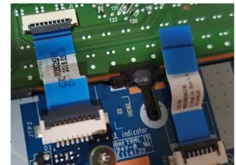
Above right: plastic strips containing wires, connected to the circuit board with connectors Above left: the motherboard
