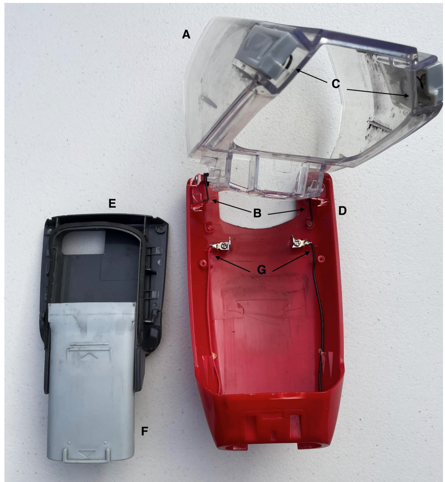
Figure 7: All the parts of the Dirt Cup (A-D and G), including the telescoping nozzle (E and F), collectively make up the front part of the vacuum.
