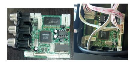
A curiosity of the digital plate is that is really sensitive, so it is the part that most problems suffers (components burn, the pins of the integrated circuits gets unsoldered and so on). We noticed that this part had all his components.
