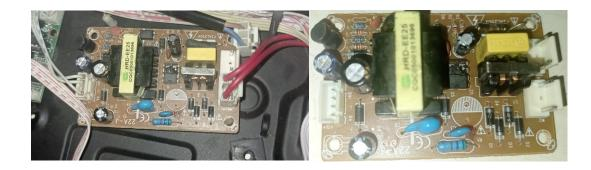
We noticed that the dvd reader didn't had 4 components (2 capacitors, a resistor and a diode), so when i tried to turn it on, it sparked and broke down
