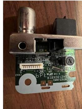
AM radio loop antenna connector
