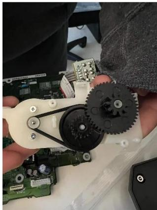
Mechanism for sliding out cover
