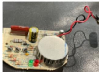
When we finally broke open the smoke detector we saw the motherboard. There were a lot of components but some of them we could already recognize. Some that we knew were the heat sync, the battery, and the sensors. Some of these looked like they were duplicated all around the motherboard. Some of the parts that were duplicated all over the motherboard were the resistors.
