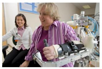
"For the NIH-funded UCI study, control software used in this robotic exoskeleton will be adapted for a compact, portable device to help stroke patients with at-home hand exercises" (Anna Lynn Spitzer).
