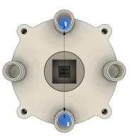
added in a circle with a radius of 0.5 inches so that the gearbox will fit on 1x3x1 and 1x5x1 C-Channel. The powered axle goes into the casing side for a torque ratio or can be put into the cap for a speed ratio.
