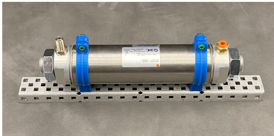
Figure 8.3. Printed mount with reservoir on C-Channel
