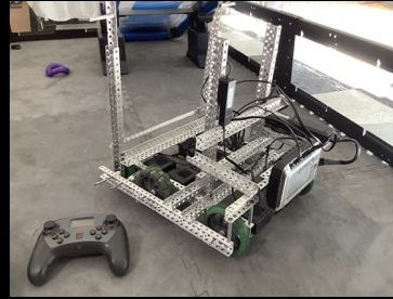
V1: Forklift with 4 omni/2 traction drive
