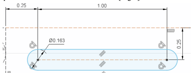
Fig 5. 0.163" x 1" slot spaced 0.25" from the top and left of the C-Channel.
