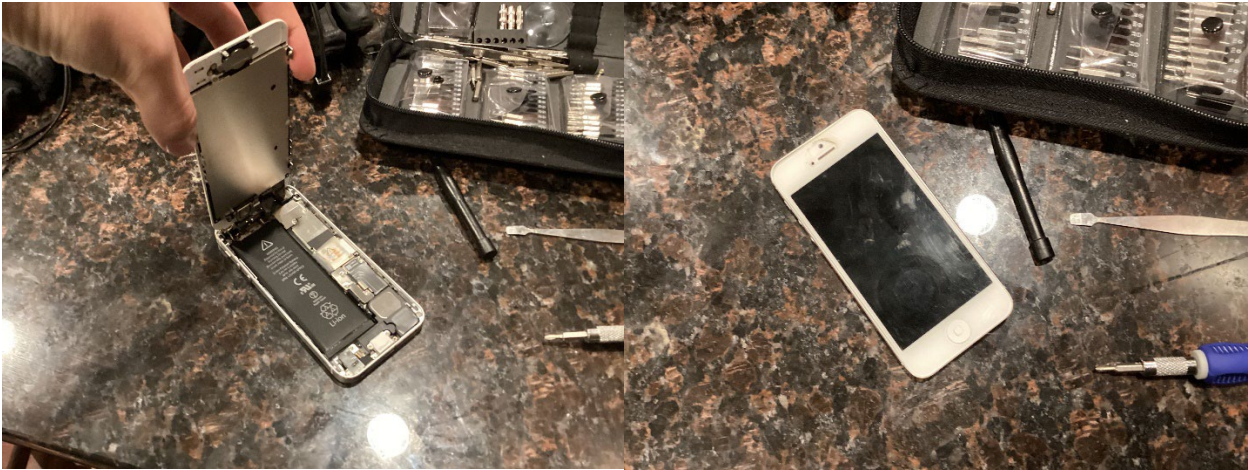
first look inside the phone and removal of phone screen.
