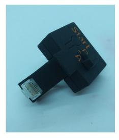
Our team designed a self-timing competition switch. It is a small box that clips onto a controller using the RJ-45 jack on the back, and a small hook that latches onto the edge of the screen. When connected, it enables the user to run a competition length timed driver or autonomous period. The user first selects which mode the switch is in. There are 3 modes. The first is marked with a D, and this
