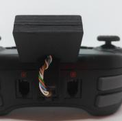
a guiding rail, to create extra bodies which filled in the gaps and fixed our issues. We also wanted some markings in a different color on the face of our switch. To do this, we designed them as a seperate component, which we then exported as a single mesh. Once we had that, we sliced the Gcode for both the main body and the markings, then modified the Body Gcode by adding a filament change call after the first layer. We then printed the 2 layers of color for the text, and changed back to
