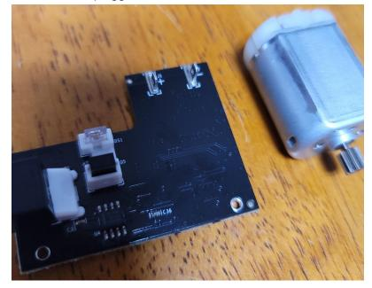
The motor itself is a brushed motor, meaning it contains two magnets each facing the center with opposite poles. Within the center is a conductor that runs up then back down,
