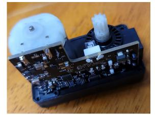
In order to fully remove the motor and circuit board, remove the bottom shell, revealing gears that go from the motor to the shaft. This set is composed of three gears with a 17:5 ratio.
