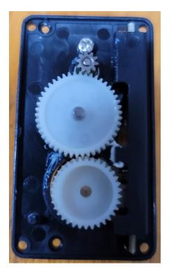
After removing the central gear you can remove the motor and circuit board from the shell. Then the motor can be unplugged.
